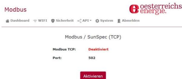
The screenshot shows the 'Modbus' configuration page. At the top right is the 'oesterreichs energie' logo. Below it is a navigation bar with links: Dashboard, WIFI, Sicherheit, API (selected), System, and Abmelden. The main heading is 'Modbus / SunSpec (TCP)'. The configuration is as follows:
